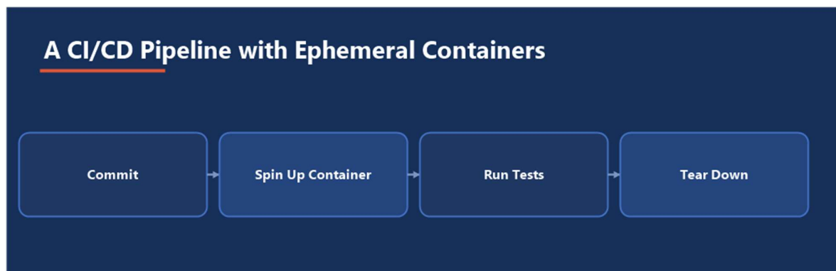
Figure 8 — Every run gets a database with no memory of the run before it
