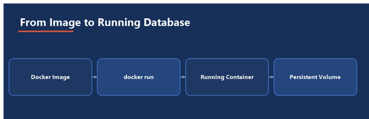
Figure 1 — The container is disposable; the volume is where the actual database lives
